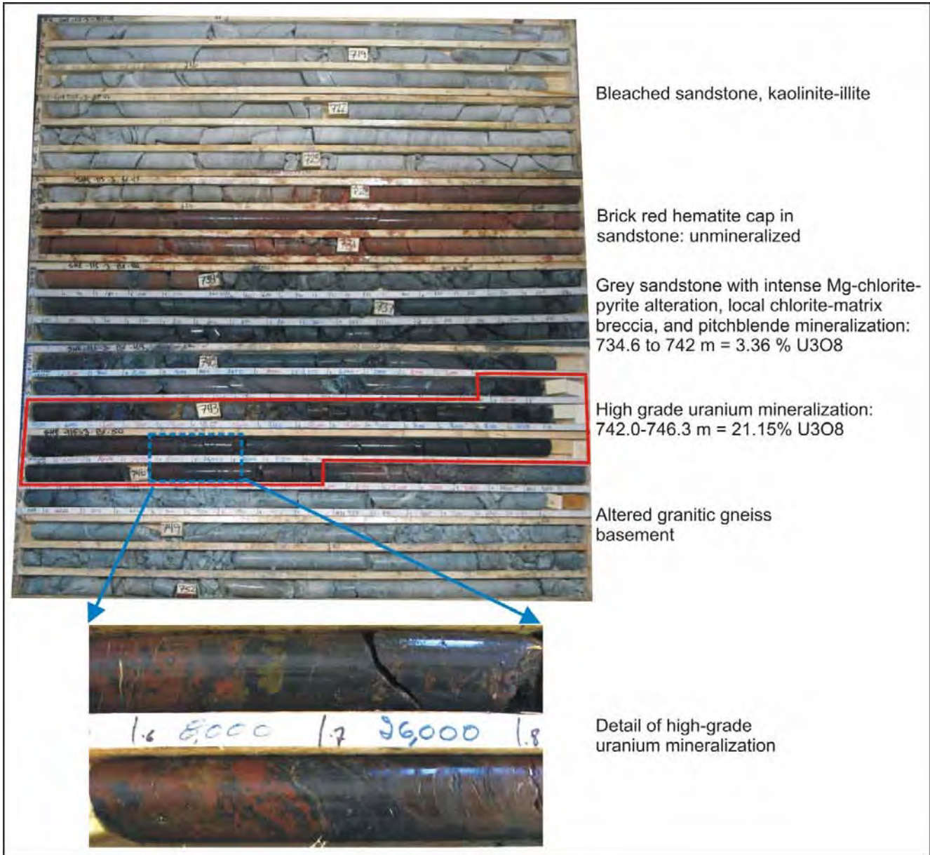
Photo 2: High-grade Unconformity Uranium Mineralization from Drill Hole SHE-115-03 in the Kianna Deposit Illustrating Textures and Associated Alteration
