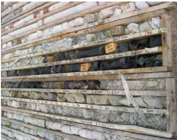
6A: Oblique view of core: black, mineralized interval is from 679 to 689 metres, and has some core loss
