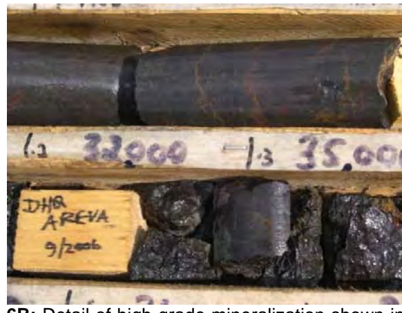
6B: Detail of high grade mineralization shown in Photo A
