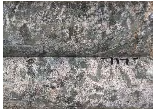
E: Amphibolite unit: Top: HS-02, 153 ft; Bottom: LB- 52, 717 ft
