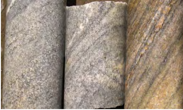
A: Arkosic quartzite unit: Left: HS-48, 348 ft Center: HS-17A, 867 ft; Right: HS-17A, 473 ft; Note pegmatite stringer parallel to foliation
