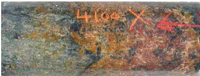
E: RU-118, 118.2 m; from interval grading 0.63% U3O8
