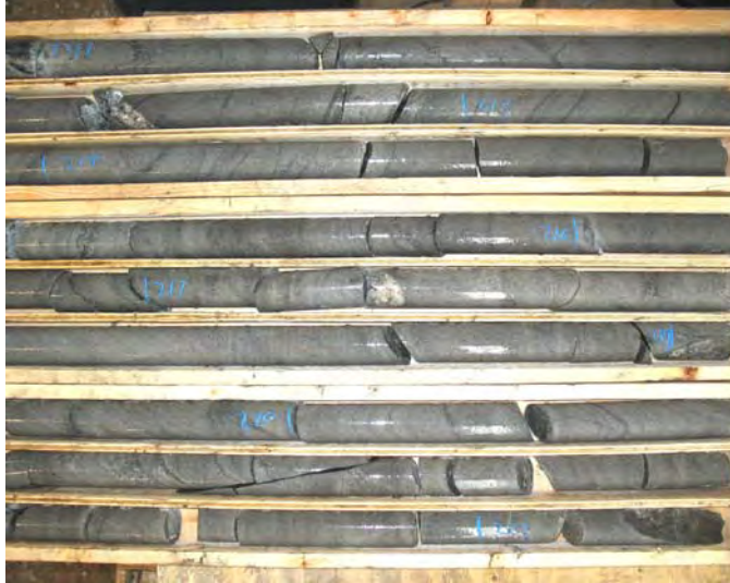
B: HU-063, 211-233 m, typical fresh arkosic quartzite
