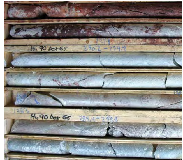
C: HU-090, 277-287 m, clay altered arkosic quartzite
