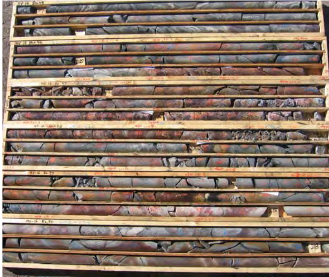
A: HU-016: entire mineralized A zone intercept, 194-219.5 m
