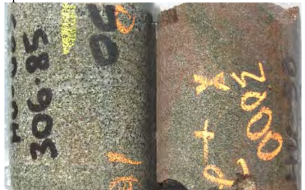
C: Left: HU-085, 306.85 m (in interval grading 0.51%); right HU-050, 308.3 m (in interval grading 0.403%)
