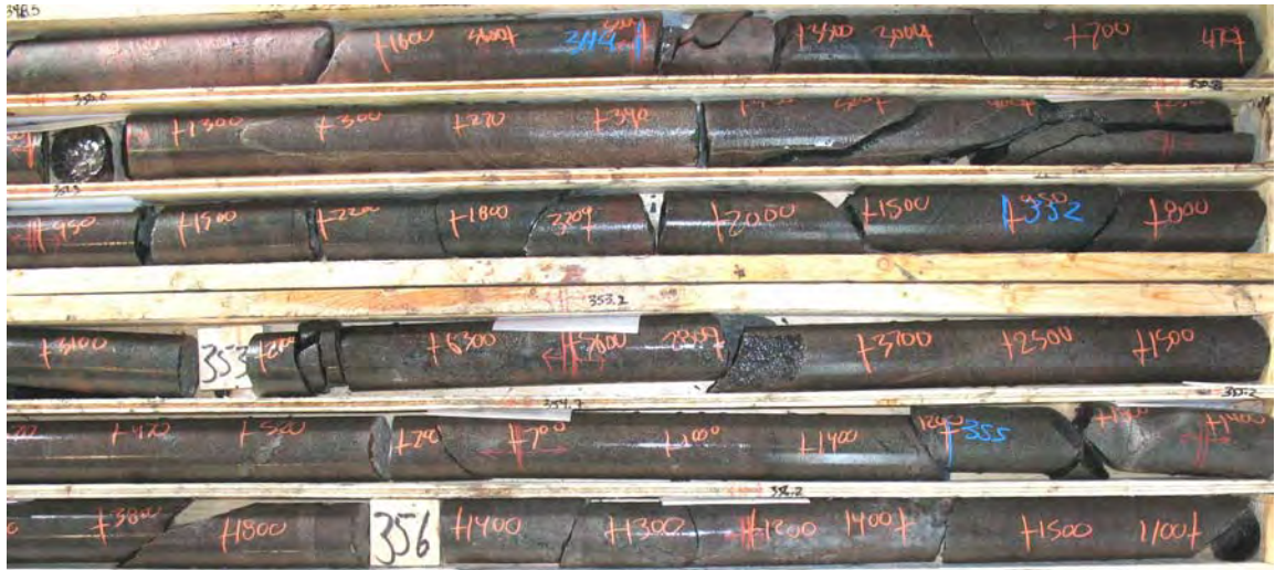
A: HU-063, 348-357 m, typical core from intercept of 0.18% over 60.90 m
