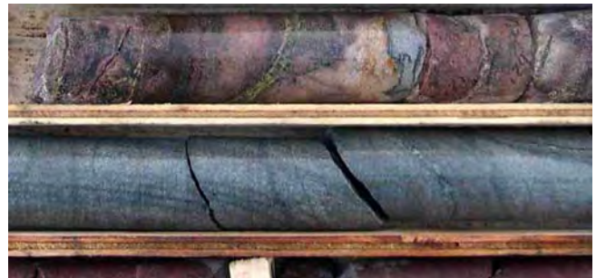
F: HU-028, 195-198.5 m. Top core = 1.23%; bottom core row = 0.055 to 0.22 % U 3 O 8
