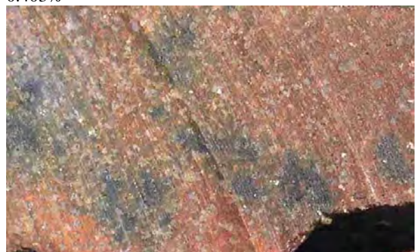
E: HU-088, 324.2 m (from interval grading 1.46% U 3 O 8 ). Field of view is 4 cm.
