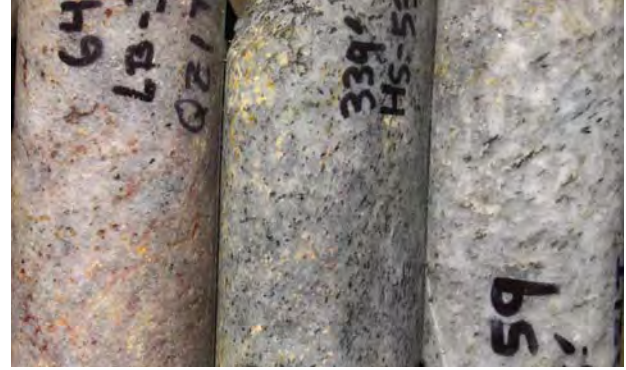
B: Quartzite unit: Left: LB-039, 640 ft (oxidized sample in alteration); Center: HS-053, 339 ft; Right: HS-059, 275 ft
