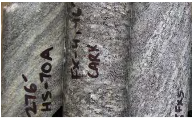
C: Upper calc-arkosic gneiss: Top photo: Left: HS- 070A, 276 ft; center: FX-04, 46 ft Right: FX-05, 198 ft
