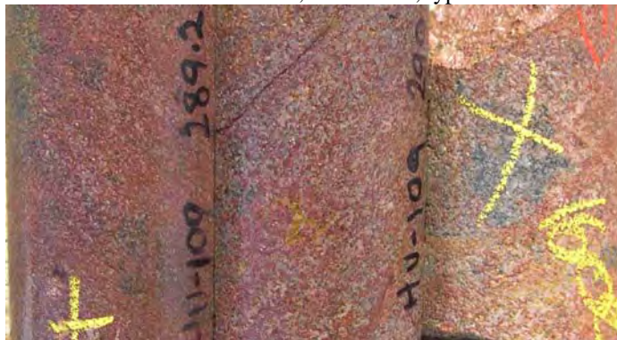
B: HU-109: core from 289-291 m (from 0.18 % over 50.1 m); samples here are from intervals grading 0.42-0.77%
