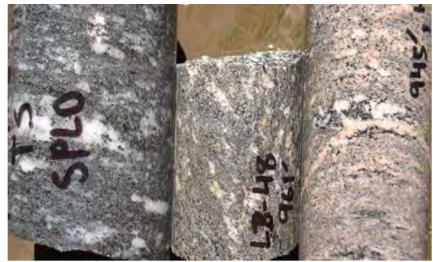
D: Semipelitic biotite-feldspar-quartz gneiss: Note deformed feldspar aggregates that may represent relict porphyritic textures. Left: HU-117, 414.6 m; Center: LB-048, 961 ft; Right: HS-089, 945 ft
