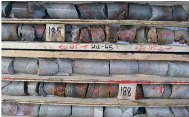
C: HU-045, 183.4-189.5 m; 185-185.2 = 5.43%; top rows = 0.01 to 0.44%; second row from bottom (187.6-188.1 m) = 0.913%
