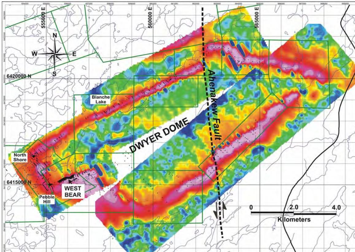
Areas in red and purple represent most conductive lithologies, outlining an elliptical rim of graphitic conductors which surround the Dwyer Dome. Property outlines are in green, and Highway 905 is the line to the right.
